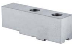
A09 Top jaw AB, special length, soft, 16MnCr5, DIN 6350
